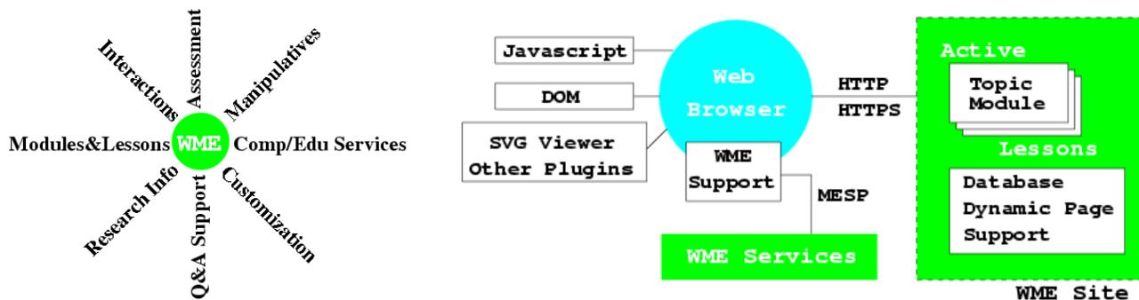
Figure 2: WME Integration (left) WME Architecture (right)
